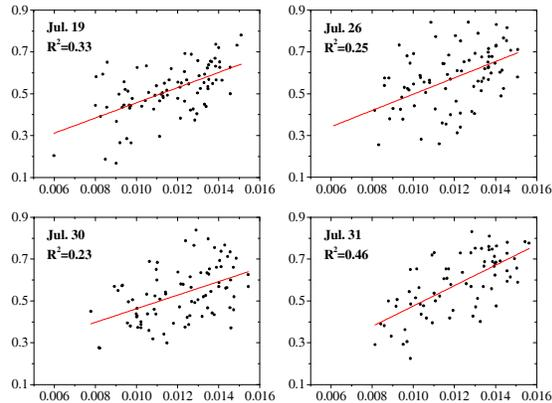
**Fig. 5.** Validation of TRVDI (y-axis) with AMSR-E PR for cloud free days in July.
