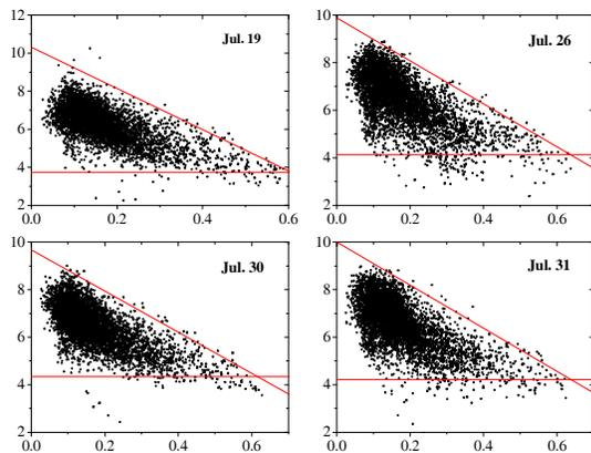
**Fig. 3.** Scatterplot of Vegetation Cover (x-axis) and Mid-morning temperature rising rate (y-axis, K/h) for cloud free days in July.
