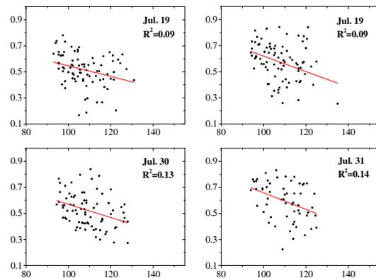
**Fig. 4.** Validation of TRVDI (y-axis) with AMSR-E surface soil moisture content (x-axis,  $0.001\text{gcm}^{-3}$ ) for cloud free days in July.
