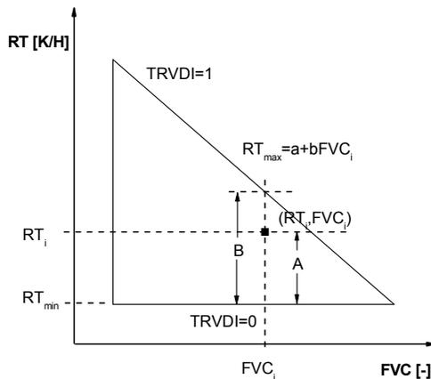
**Fig. 1.** Definition of the TRVDI. For a given pixel  $i$  ( $NDVI_i$ ,  $RT_i$ ), TRVDI is estimated to be the proportion between lines A and B
